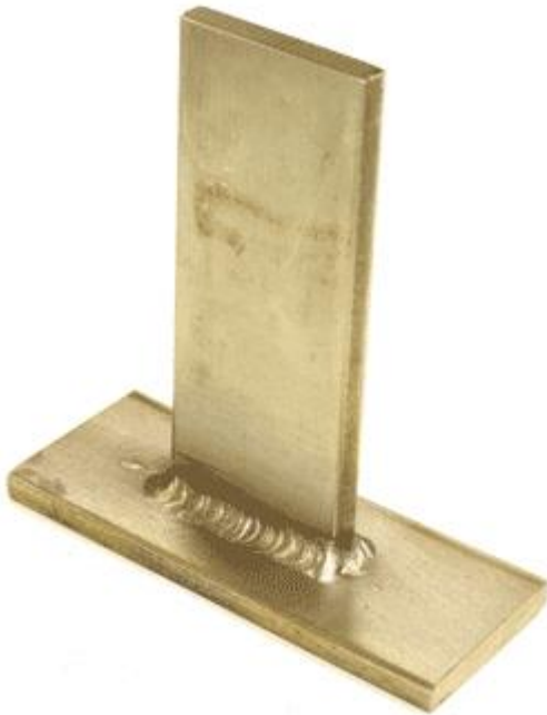
A Fillet weld made on the course
