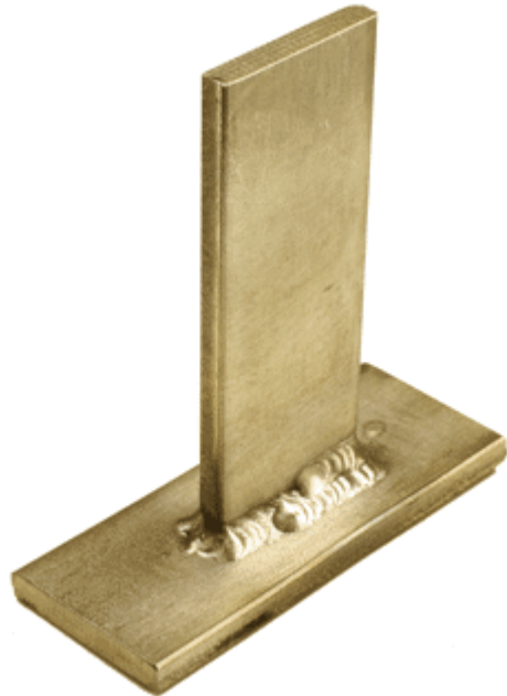
A Multipass Fillet weld made on the course
