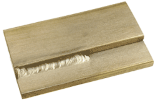
A Lap weld made on the course
