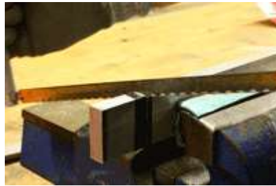
Candidates sawing off the base of the V Block
