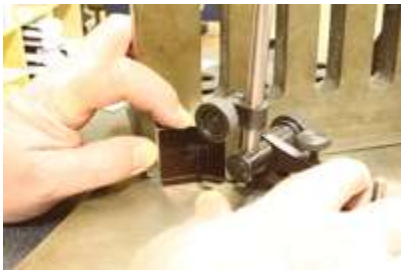
Candidates marking out the first part of the V Block
