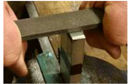
Candidates filing off square the bottom part of the V Block
