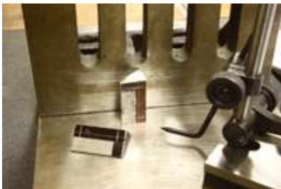
Candidates marking out the position of the holes in the V Block
