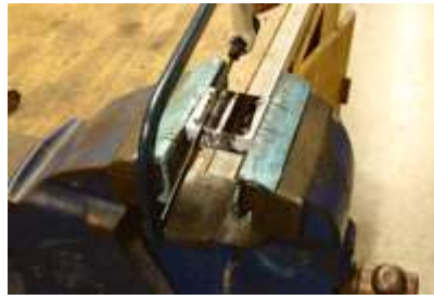
The bottom part of the V Block being channelled out using saws and files
