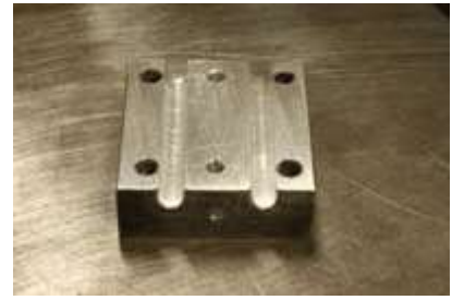
The finished bottom part of the V Block
