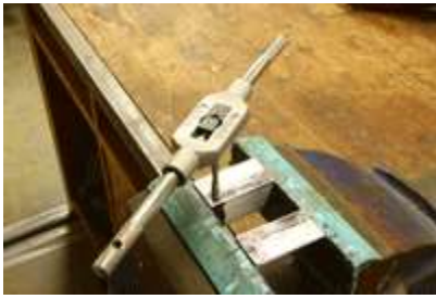
The upper parts of the V Block being threaded
