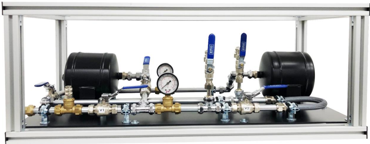
Practical rig No1 used, helping candidates gain meaningful practice of line breaking pipework isolation procedures
