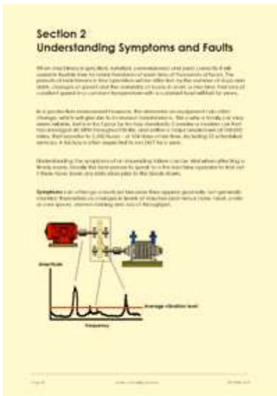
Page 12 of the course notes, where we teach the candidates about fault finding on industrial machines, thinking about symptoms, faults and causes
