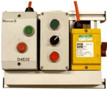
One of the isolators used to explore the correct isolation procedures necessary for safety
