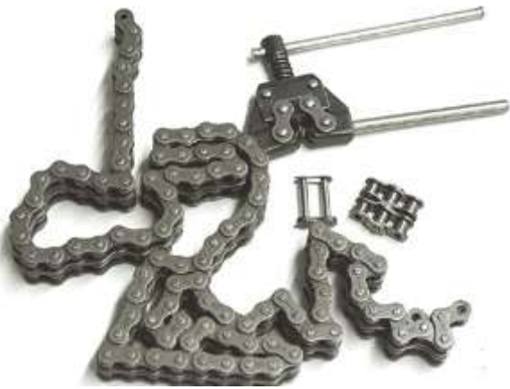
Candidates are provided with a range of chains - they insert or remove links using special tools
