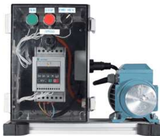
The Siemens training rig: a real industrial drive connected to a real 3-phase motor so that candidates can explore the effects of changing parameters on the Siemens drive
