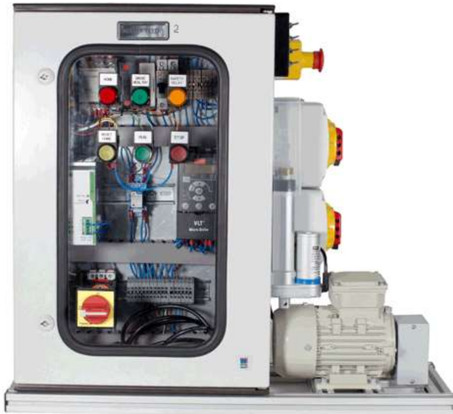
One of the motor control panels that candidates on the electrical problem solving course use
