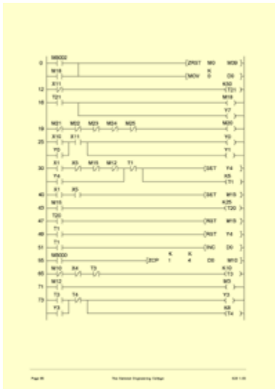
Page 60 of the PLC training courses notes, presenting the ready-written Mitsubishi PLC program
