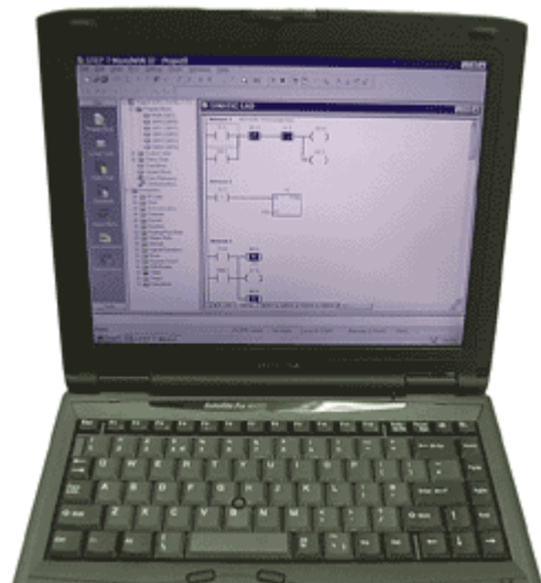
The Siemens Step 7 PC-based software package used on the PLC training courses
