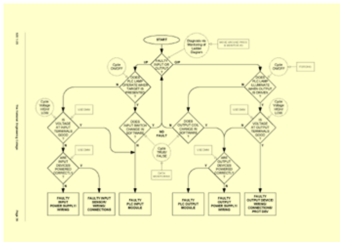
Page 39 of the PLC training courses notes, depicting the flowchart that we advocate for fault finding in PLC controlled systems
