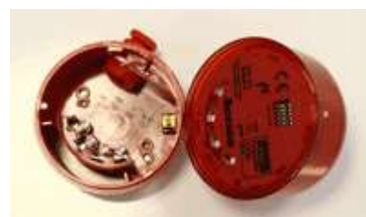
Some of the detector bases, Manual Call Points (MCPs) and sounders used as demonstration pieces for the candidates to look at on the fire alarm system training course
