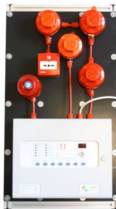
Conventional 4-Wire System 1 used on the fire alarm system installation training course
