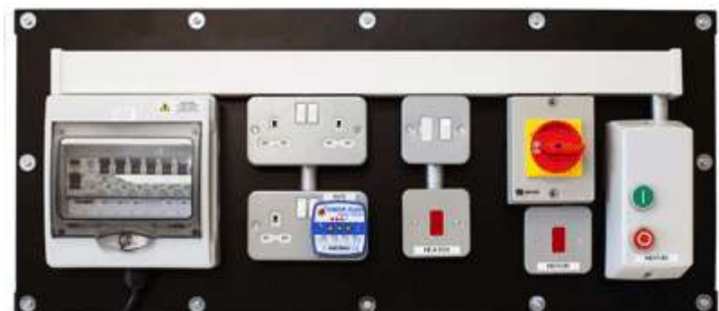
This is one of the units that are used to check that the candidates are able to isolate a single-phase system.
