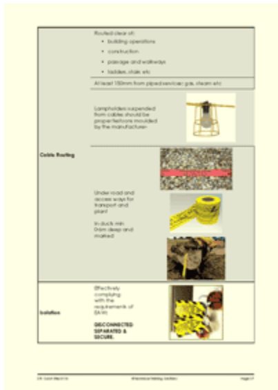
This is the page 37 of the course notes for the BS7375 course, showing what sort of lampholders are required, how underground cables should be marked and the importance of proper isolation procedures
