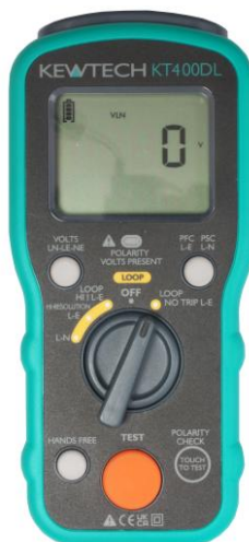
One of the earth fault loop impedance testers used on the course
