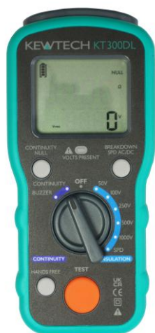
One of the continuity and insulation resistance testers used on the course
