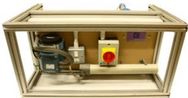
The single phase training rig. This is mains powered so the candidates have to safely isolate the heater then open the appropriate covers to get to the necessary terminals. They can then conduct the inspection and testing.
