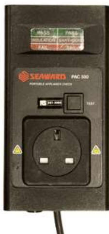
One of the PASS/FAIL types of PAT testers used on the PAT testing training course
