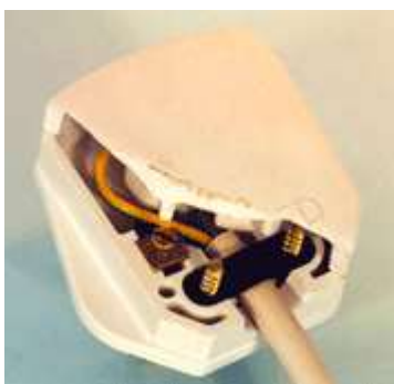
One of the pictures of a faulty plug-top used on the PAT testing training course
