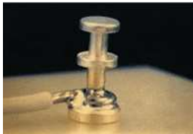
Examples of how terminal pins should be soldered to the IPC610 Standard are provided on the soldering course
