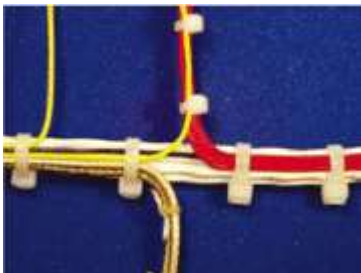
Examples of how cables should be formed to the IPC610 Standard are provided on the soldering course
