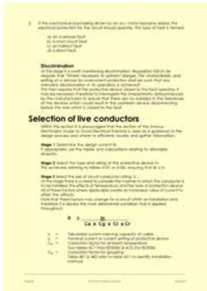
Page 28 of the 17th edition IET Wiring regulations training course notes: examining the equations used to specify the tabulated current ratings of the cables needed for a given circuit
